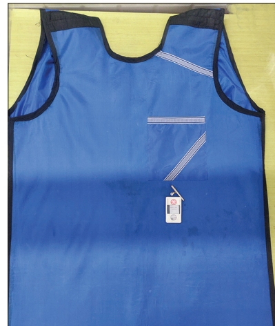
Figure 2: Thermoluminescent dosimeter (TLD) in radiology apron.
