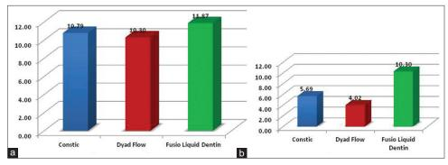
Figure 1: Graph showing (a) Mean tensile bond strength in MegaPascals (MPa) (sound enamel) and (b) mean tensile bond strength in MPa (demineralized enamel).
